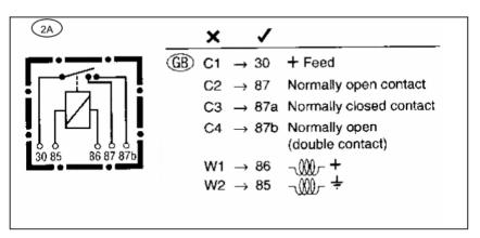
So how do I hook up the new cube-shaped relay? The bottom of the relay (3A) is shown with the modern as well as the old terminal designations. You will need to refer to the
